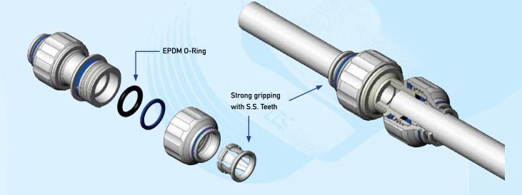
Ensure that the tubing is pushed into the fitting fully past both the collets [gripper] and the 'O' ring and is engaged properly in accordance with the manufacturer's instructions.
