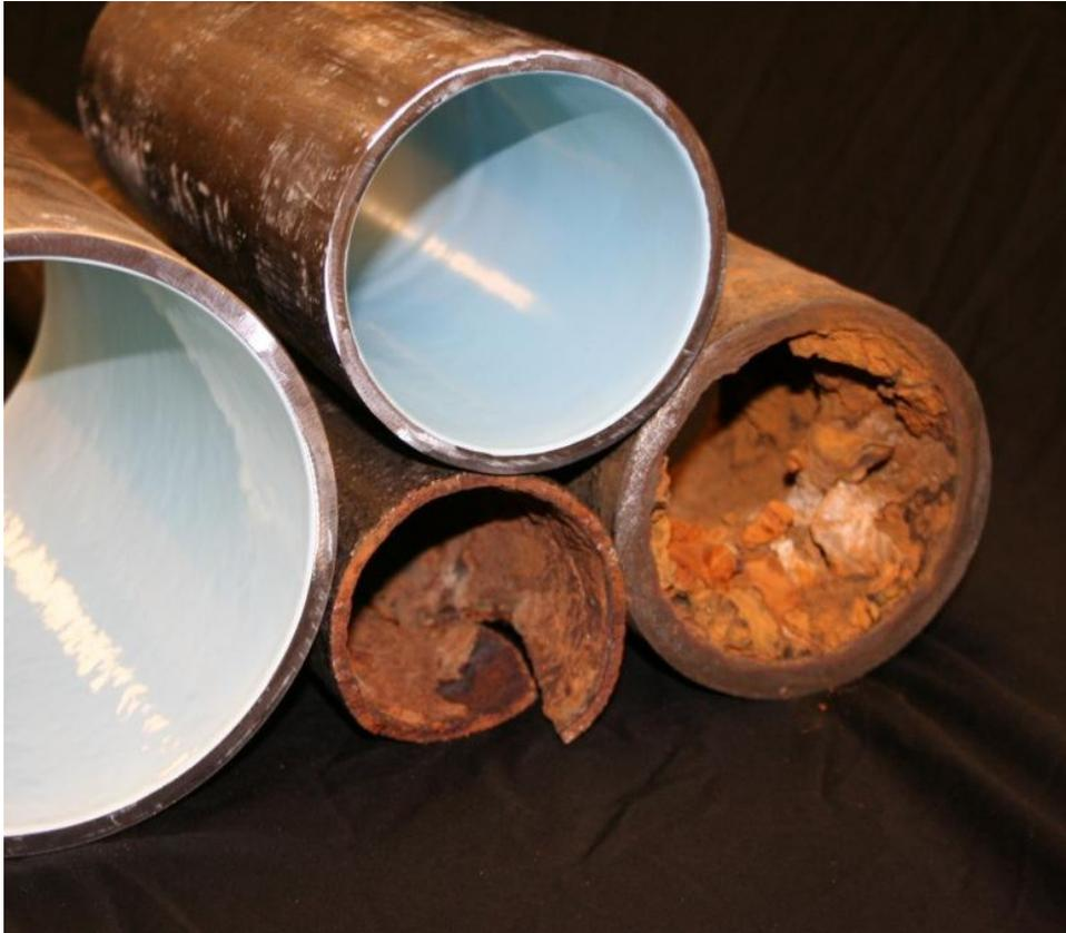
*<<<< These are new water pipes on the left that are being used to gradually replace the older crud laden water pipes on the lower right.*
